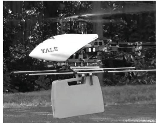
(b) Yale University's miniaturized helicopter, endowed with a gripper, transporting a load.
