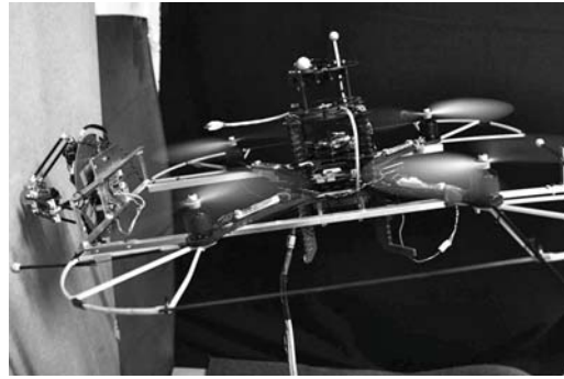
(b) The Asctec pelican's quadrotor, endowed with a robotic manipulator, in interaction task.
